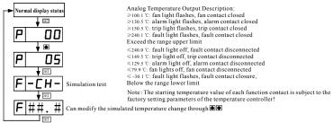
Factory function setting: during the simulation test, the overtemperature trip functioncontact is started by default; If the simulation test requires the overtemperature trip function contact point not to start, can be set according to point 3.6.
